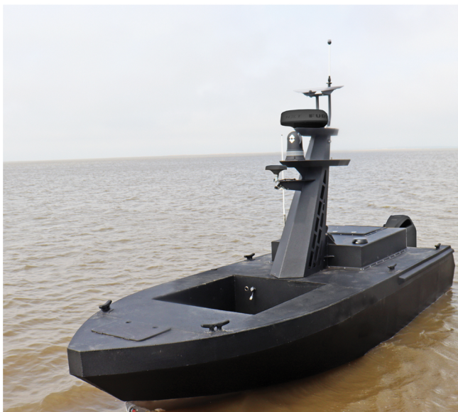
HSMUSV's forward and aft payload bays can support tethered or untethered UAV systems, surveillance or munitions systems, or organically explosive charges
